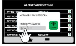
c) Use the alpha numeric keypad to enter the password and after finished press the button  $\frown$ .
