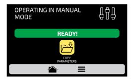
f) Copy Parameters enables the user to transport the parameters set in Manual Mode for the Edition of Groups and Recipes, that is, when click on the icon  $\swarrow$ , it will be necessary to inform the user's access password to the settings.
