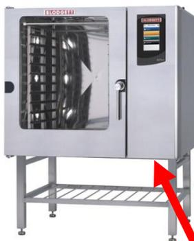
**Q1 Cavity High Limit-** is on the left. Fix problem before resetting. Unscrew and remove the cap. A very small screw driver or paper clip is needed to push up inside to reset. Unplug the oven before resetting.
