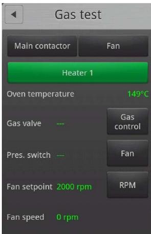
2. On the **Technician** menu, touch **Test** functions, and then touch **Gas**.
