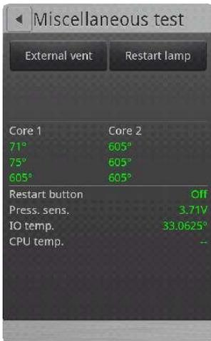
1. On the **Technician** display, touch **Test functions**, and then touch **Miscellaneous**.
