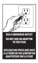
If the power supply cord is too short, have a qualified electrician or serviceman install an outlet near the appliance. Consult a qualified electrician or serviceman if the grounding instructions are not completely understood, or if doubt exists as to whether the appliance is properly grounded.
