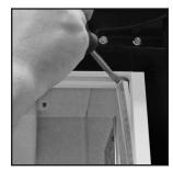
Pry the screwdriver between plastic lens cover and cabinet frame.
