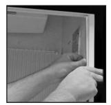
Attach wires, observing color coding. Press lens cover back to cabinet frame.
