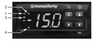
At the left side of the controller display are the following LED indicators:
