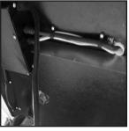
Locate the wire for the LED strip in the electrical box and disconnect from connectors.
